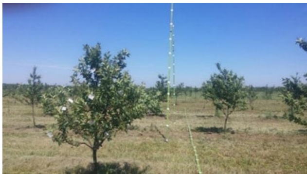
Figure 2 Drift and deposit measurement in orchard
