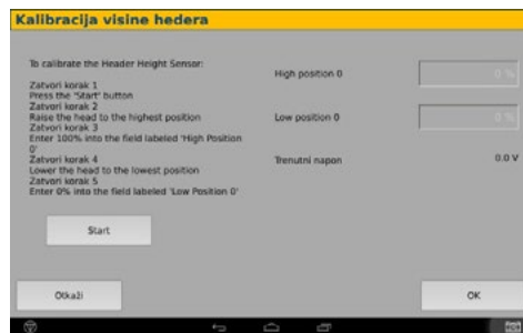
Figure 13. Header height calibration
