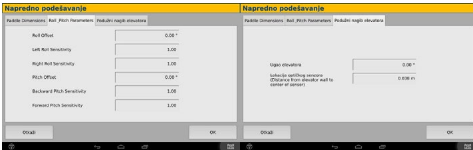
Figure 9. Entering the value of the elevator angle and its compensation
