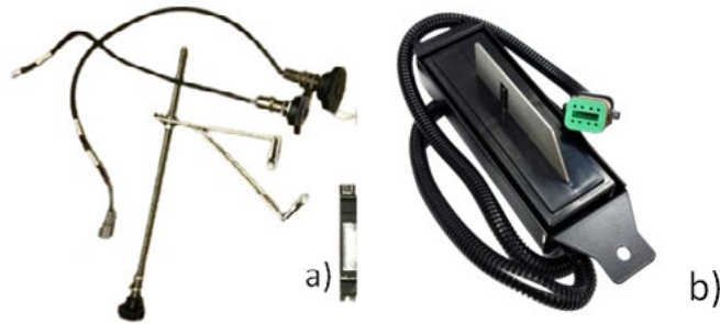
Figure 1. (a) Optical sensor that measures the fill level at the blades of the mass elevator (b) Ag Leader moisture sensor
