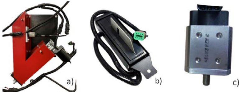
Figure 3. (a) Moisture measurement system (b) moisture sensor (c) header height sensor
